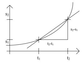
$$v = \frac{s_2 - s_1}{t_2 - t_1} = \frac{\Delta s}{\Delta t} = \tan \alpha$$
